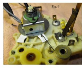
clearly. A replacement was made from suitably thin plastic.
