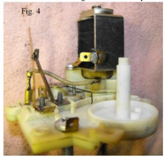
that had been sucked into valve and was caked around the plunger seal stopping it seating properly and thereby leaking air into the system
