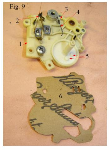
happens the plunger will not return to its closed position allowing air into the system which will upset the carburetion when the engine is idling. The dirt allowed into the system may
