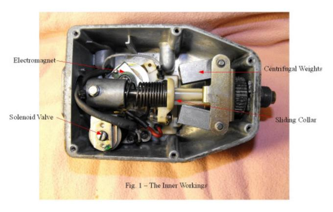
Once on the workbench remove the six screws securing the top cover which lifts off to reveal the inner workings (Fig.1).
